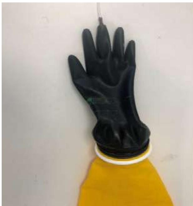
Figure 1: Placement of the pressure hose on the fingertip
